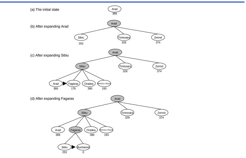
Stages in a greedy best-first search for Bucharest using the straight-line distance heuristic  $h_{SLD}$ . Nodes are labeled with the *h*-values.
